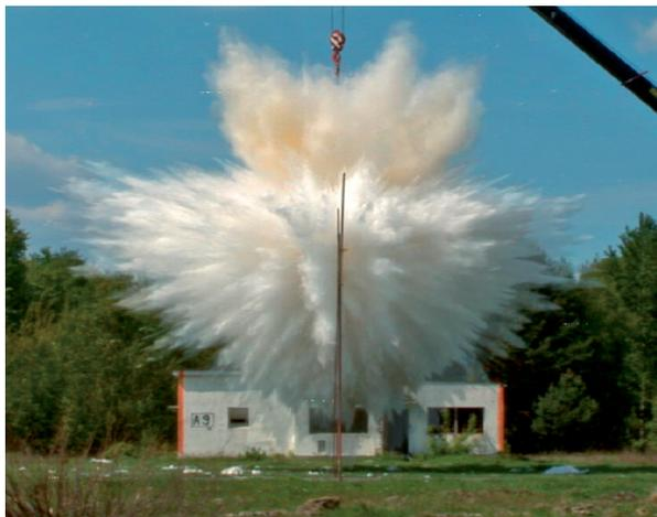
**Figure 2.** The explosively developed water-spray cloud.
